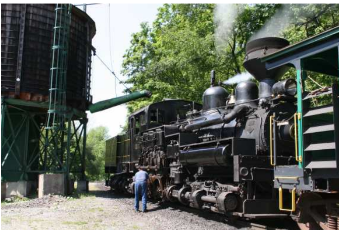
Topping off the water and checking the drive train before backing into the station for departure. Photo by R. Lind.
