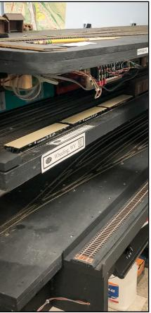
three staging yards are similar for each yard. Each panel has a rotary switch to choose the proper staging track. This makes picking a staging track pretty straight forward for my operating crews at the Pittsburgh & South Pennsylvania (P&SP) RR.
