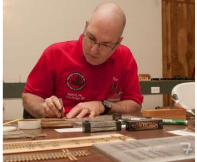
Ken Mazer – Hand laying turnouts using Fast Tracks jigs
