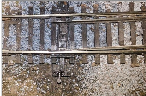
Above is a picture where the magnets are contacting the pin [*Attached magnets are only on the lower side of the throw bar for illustration purposes. - Ed.J.*]
